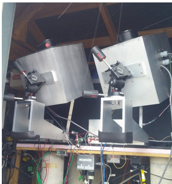
Figure 1: The EMCCD CAMO array at the Elginfield Observatory, consisting of two Nüvü HNü EMCCD cameras with attached 75 mm lenses, pointed at a common field.
