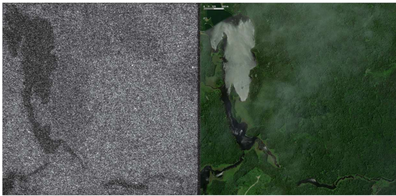
Figure 1 Left: Nighttime nüSpace EMCCD ground image in starlight conditions taken with f/11 optics using 1 fps standard snapshot imaging with EM gain; Right: Comparative satellite daytime ground image.
