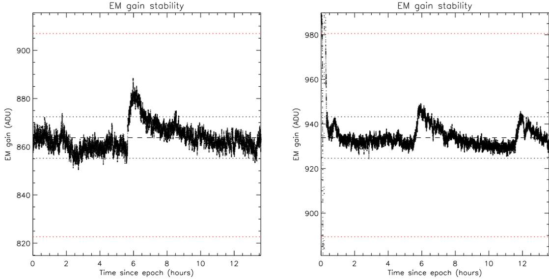
Figure 12: High gain stability. **Left:** SN1. **Right:** SN2. The red dotted lines represent a  $\pm 5\%$  variation, and the black dotted lines a  $\pm 1\%$  variation over the median.
