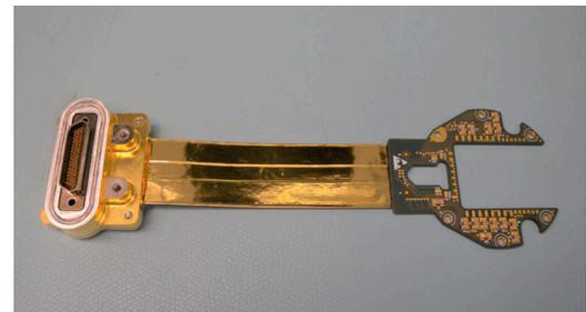
Figure 5: CPE's EMCCD headboard, showing the custom backshell and the gold tape on the flexible portion.
