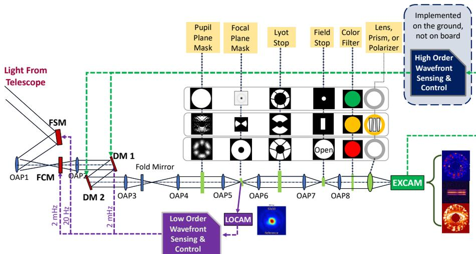
Figure 1: The CGI mechanical (**top**) and optical (**bottom**) concepts, showing the location of the LoCam and ExCam (circled in red). Figures taken from [1].
