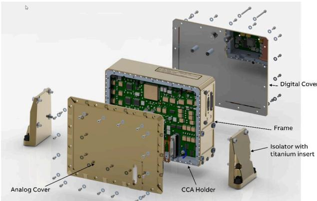
Figure 4: Exploded view of the CPE enclosure.
