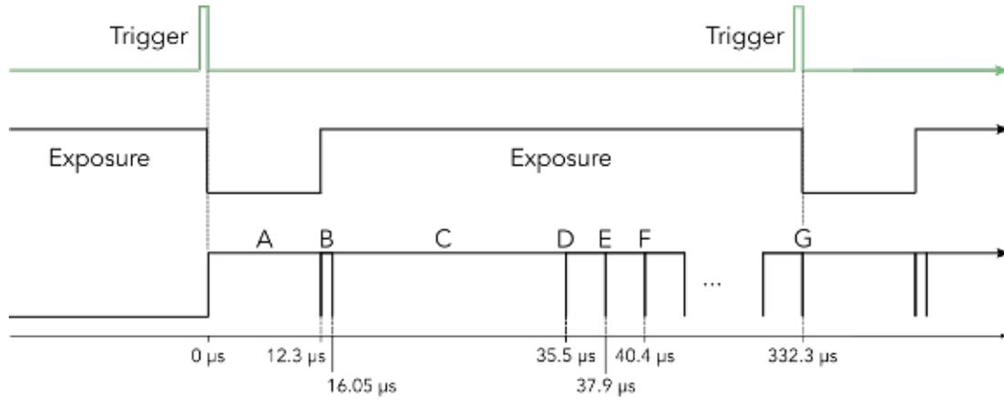
A- Frame transfer    B- ADC latency    C- Pipelining    D- 1<sup>st</sup> pixel
