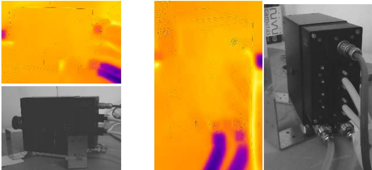
Figure 5. Thermal imaging showing the camera and the water circuits that are 3°C below ambient. Corresponding visible light images are shown as a reference. **Left:** Side of the camera, showing a very uniform temperature on the camera body and no difference with respect to the ambient furniture. **Right:** Back of the camera, emphasizing the water circuit and the power cord (warmer than the body).
