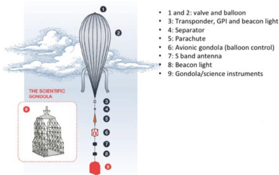
Figure 1. Typical stratospheric balloon components (from CSA website).
