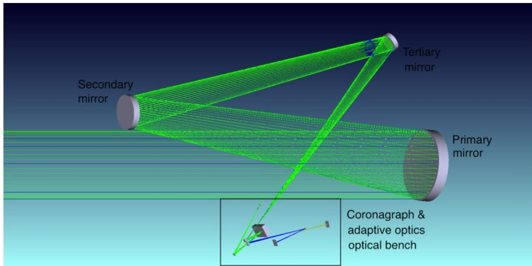
Figure 5. The overall MAPLE-50 spherical optical design.
