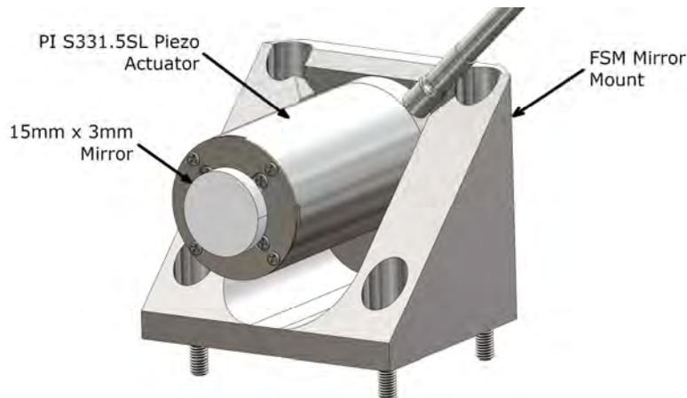
**Figure 13. FSM mount design**
