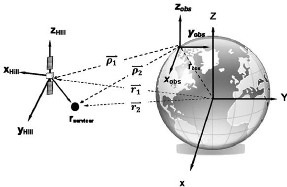
Fig. 5. Geometry of client and servicer observations.
