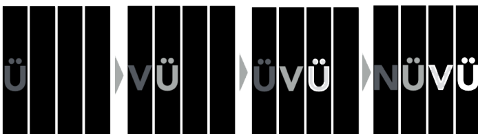
Fig 1. Example of imaging the word NÜVÜ using TDI readout mode. The intensity of the signal is increased as the word moves across the detector
