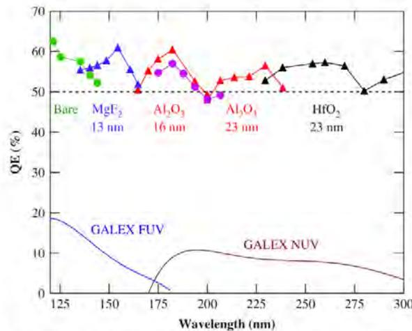
Figure 6. UV response of an AR-coated, delta-doped CCD, showing 50% or greater QE. (Credit: Nikzad et al. 2012)
