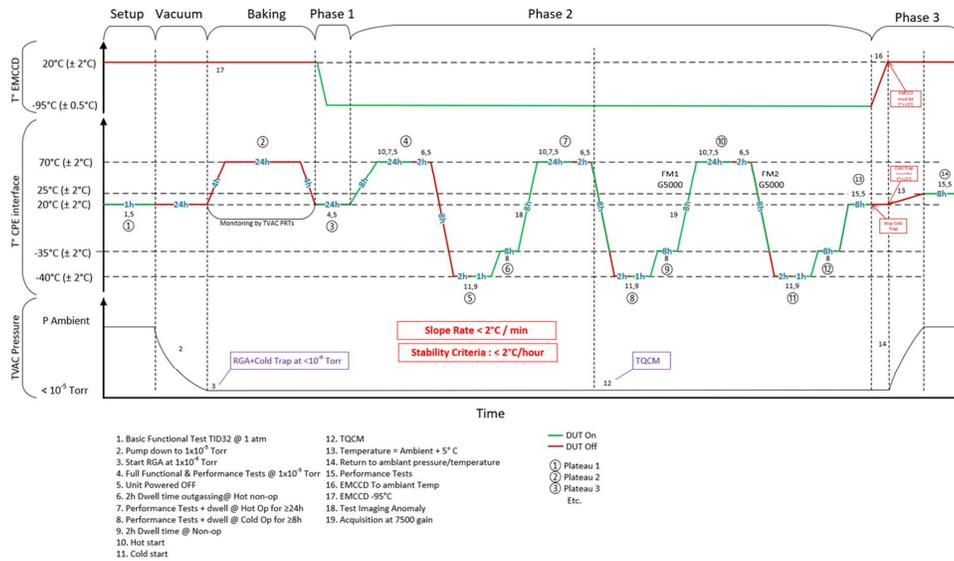
Figure 10: Pressure and temperature profiles for the TVAC campaign.
