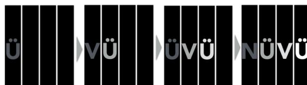
Fig. 1. Example of imaging the word NÜVÜ using Time-Delay Integration readout mode. The intensity of the signal is increased as the word moves across the detector.
