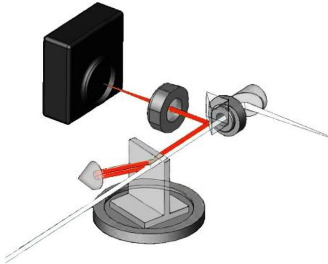
**Figure 3: Current design of a transmission imaging Bragg tunable filter using a volume hologram.**
