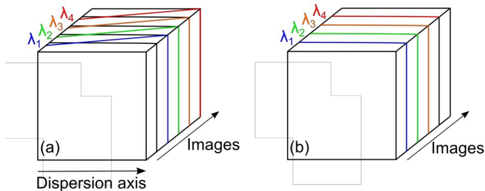
**Figure 4: (a) Images with a gradient in wavelength in the dimension parallel to the dispersion axis and (b) reconstructed monochromatic images.**
