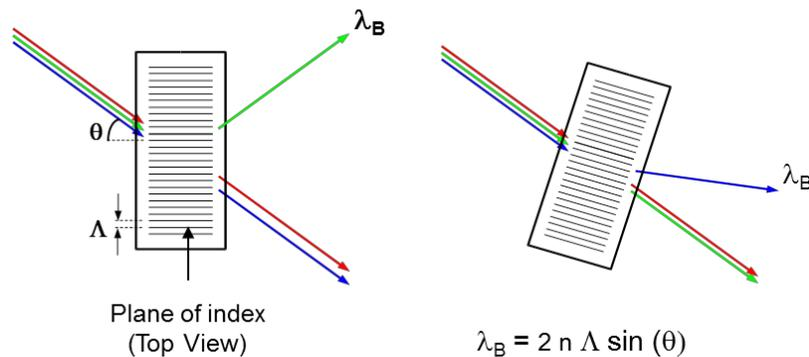
Figure 2: Filtering scheme for transmission BTF
