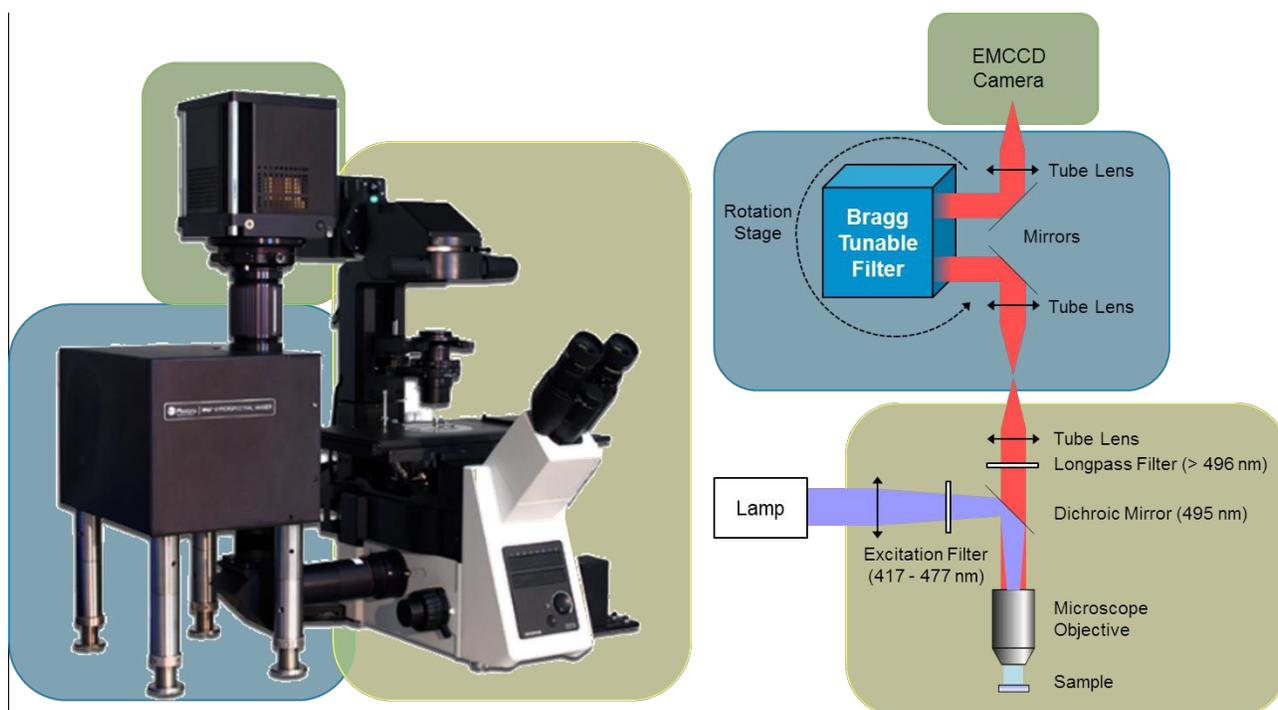
**Figure 1: Scheme of the multiplex hyperspectral imaging platform with the main components: microscope (yellow background), hyperspectral filter (blue background) and camera (green background).**
