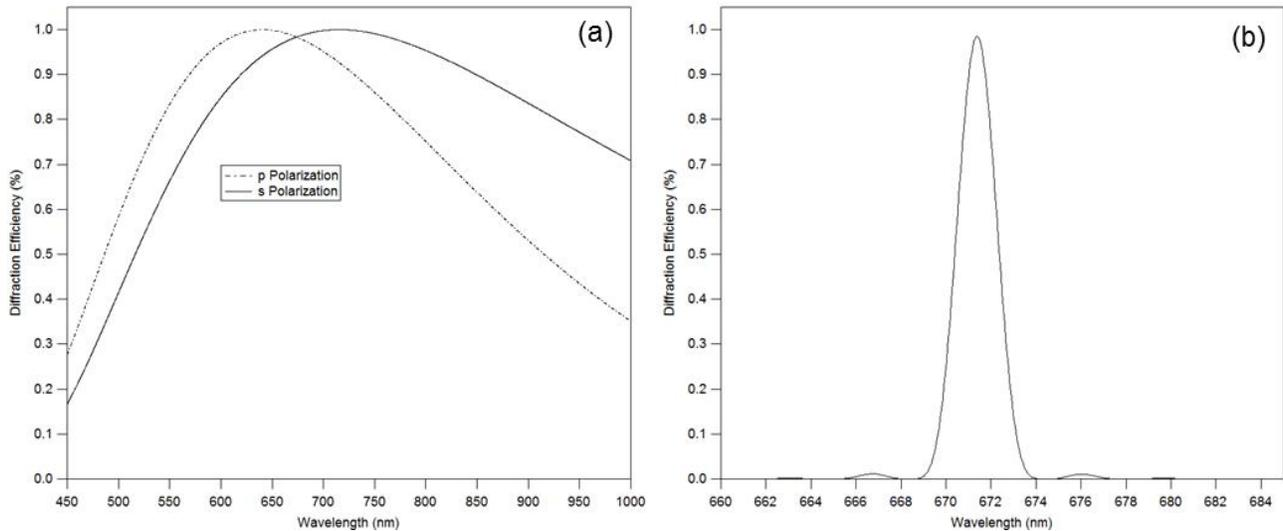
**Figure 5: (a) Modeled diffraction efficiency for a reflection volume hologram for s- and p-polarization (solid and dash lines, respectively). (b) Spectral response of the volume hologram centered at 671 nm.**
