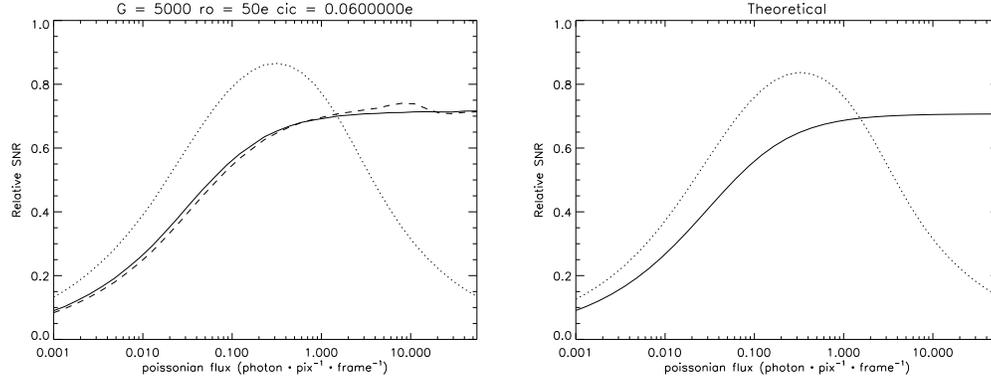
**Figure 6.** Relative SNR of a "real" EMCCD, compared to a perfect photon counting system, including the effect of read-out noise (50 electrons) and the effect of spurious charges (0.06 event/pixel/frame) at a mean gain of 5000. Left panel: result of simulations. Right panel: theoretical values. Dotted line: PC, dashed line: PP, plain line: analogic.
