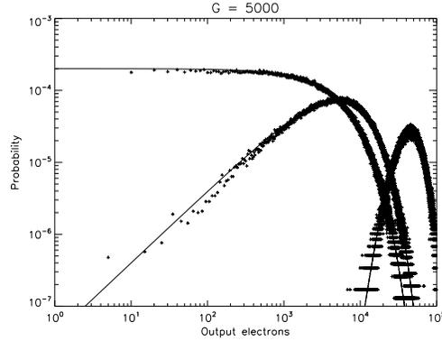
**Figure 1.** Simulated (crosses) and theoretical (plain lines) output values of an EMCCD multiplication register of 536 elements for a mean gain of 5000. The plotted values are for one, two and ten input electrons (leftmost to rightmost curve). The simulated values were binned into 10 output electrons bins. The hatched appearance of the simulation results at low probability comes from the amount of iterations of the simulations. The generation of more events would be required to overcome this.
