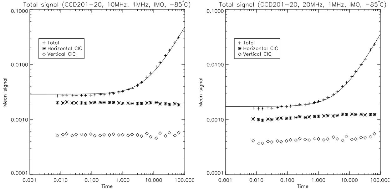
Figure 10. CIC and dark measurements at an EM gain of 1000 and an operating temperature of  $-85^{\circ}\text{C}$ , displaying the total background signal measured as a function of the integration time. **Left:** at 10 MHz. **Right:** at 20 MHz. The plain line represents a linear fit to the data.
