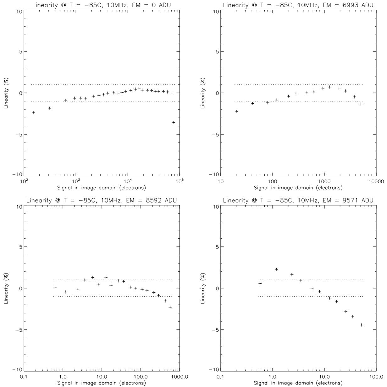
Figure 8. Linearity measurements at 10MHz, for various EM gains. **Top left:** Unity. **Top right:** 10. **Bottom left:** 100. **Bottom right:** 1000. For every graph, the linearity measurements at the lowest fluxes might be disturbed by the readout noise. The dotted lines shows the  $\pm 1\%$  boundaries.
