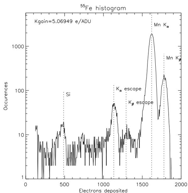
Figure 1. Images histogram of the CCD201-20 chip conventional output exposed to the <sup>55</sup>Fe source. Images were cleaned to remove shared events between two or more pixels before generating the histogram.
