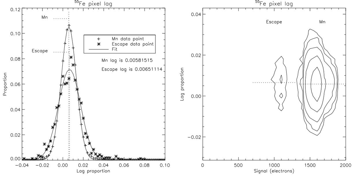
Figure 4. EM register CTE measurement at a gain of 10. **Left:** signal histogram with respect to pixel position for all Mn and escape lines isolated events. **Right:** Map of the 2D signal distribution based on the energy of the main pixel. The intervals delimited by the dotted line indicate the range of energy used for the left graphic curves (x axis) and the average signal assessed by the Gaussian fit (y axis).
