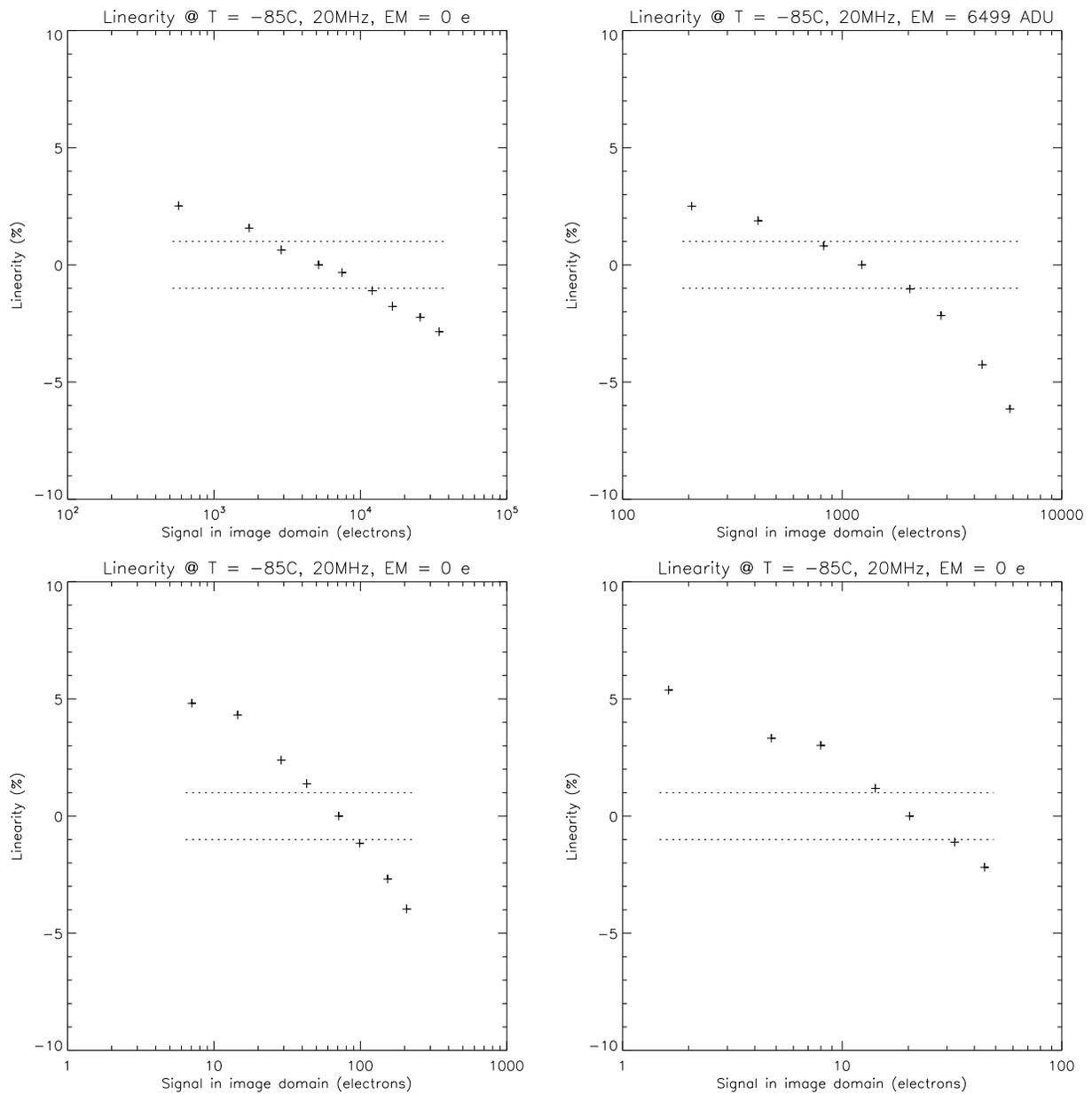
Figure 9. Linearity measurements at 20MHz for various EM gains. **Top left:** Unity. **Top right:** 10. **Bottom left:** 100. **Bottom right:** 1000. For every graph, the linearity data at the lowest fluxes might have been disturbed by the readout noise.
