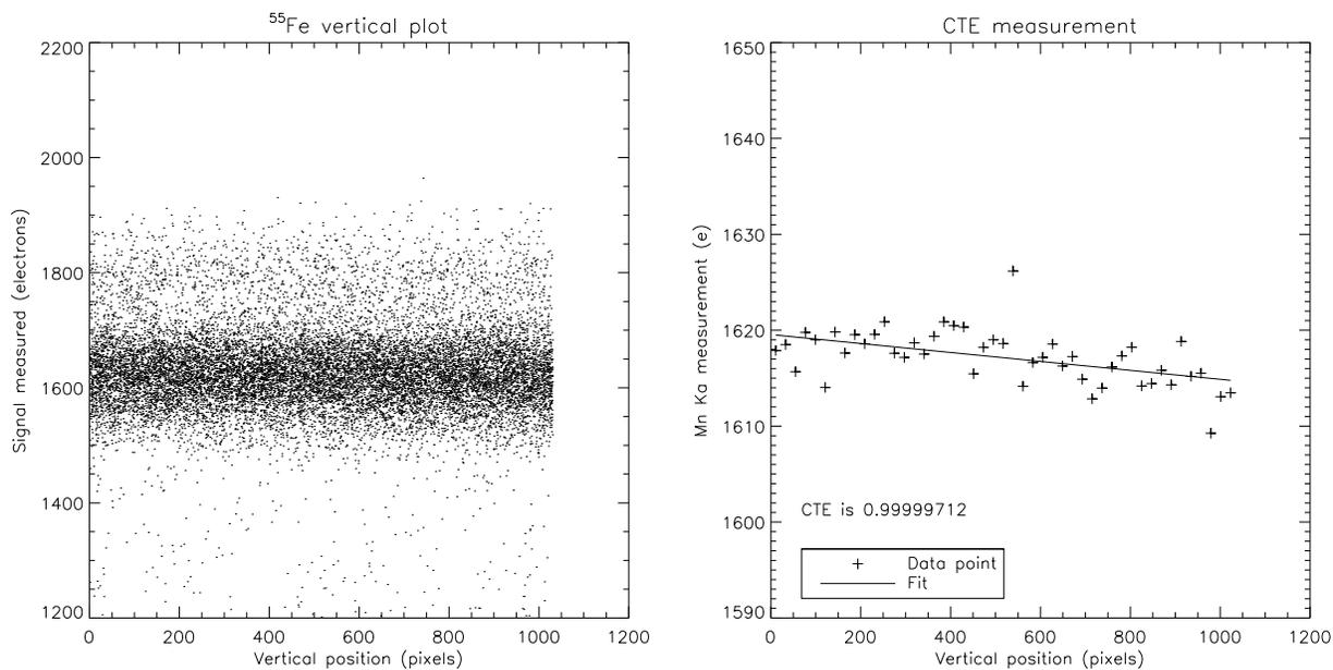
Figure 2. Example vertical CTE determination using 1MHz sinusoidal clocks. **Left:** X-ray intensity map with respect to vertical position. **Right:** CTE computation via a linear fit using the data from the left graphic with the Mn K<sub>α</sub> line.
