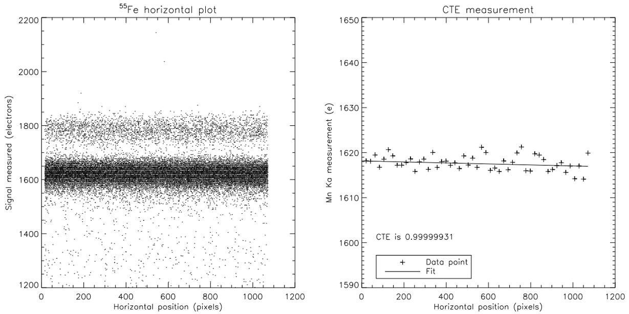
Figure 3. Horizontal CTE determination for the conventional register with a 100 kHz clock. **Left:** X-ray intensity map with respect to horizontal position. **Right:** CTE computation via a linear fit using the data from the left graphic with the Mn K $\alpha$  line.
