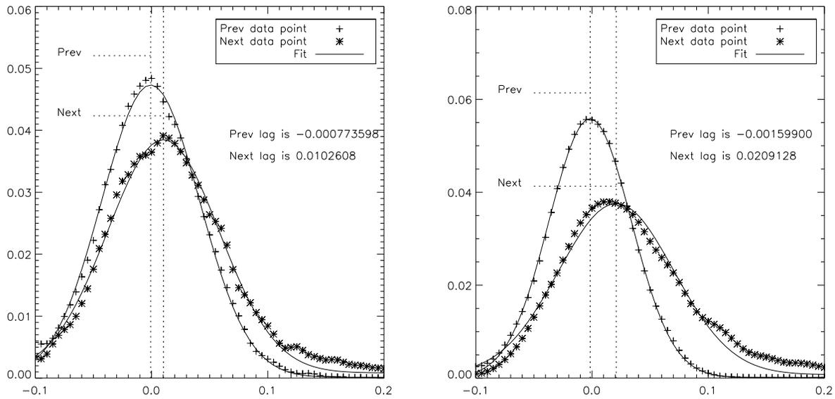
Figure 7. Measurement of the deferred charges for the pixel previous (+) and next (\*) to a pixel of signal when operating the EMCCD at high gain (1000). The plain lines show a Gaussian fit to the data. **Left:** at 10 MHz. **Right:** at 20 MHz.
